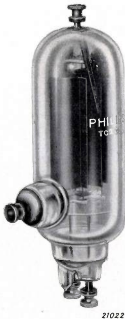
Fig. 4. The TC 2/300 transmitting valve. The anode is welded at the top to a chrome-iron plate which is fused to the bulb; at the lower end it is supported against the bulb by a mica disc. The ceramic insulating distance pieces are visible above and below the anode.
