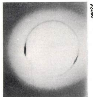
Fig. 2. The holes in the two plates of the riveted joint do not lie directly one above the other.
