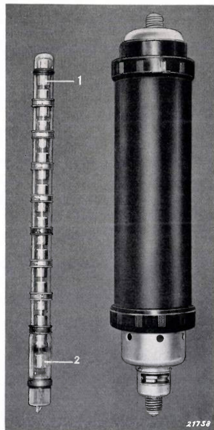
Fig. 3. High tension valves, 1 anode, 2 cathode. The path of the discharge between anode and cathode is subdivided by means of 8 metal cylinders in order to divide the inverse voltage uniformly.
