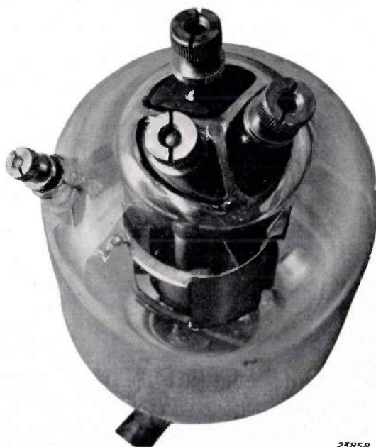
Fig. 13. Three electrodes of a rectifier valve are led in by means of sector-shaped chrome iron plates. The three plates are first welded together with a glass edge to give a circular plate and then sealed on to the circular opening of the rectifier bulb.
