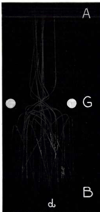
Fig. 8 a - f. Photographs of paths of balls, obtained by shooting a parallel "beam" of balls (in the arrangement of fig. 3) with a constant velocity perpendicular to the line joining the grid supports. The different figures are obtained by taking the height of G successively a little greater.
