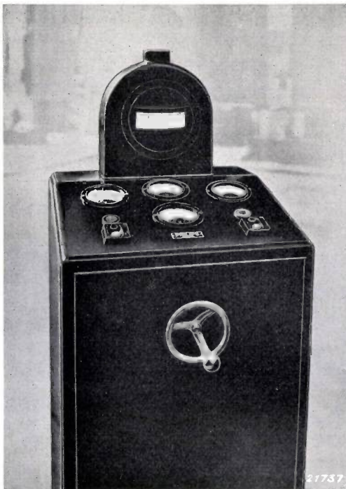
Fig. 4. Control table of the high tension installation. The excitation of the alternator which acts as source of potential, and thereby also the DC voltage reached, is regulated by means of the hand wheel. The voltage reached can be read off immediately from the vertically placed electrostatic voltmeter above.
