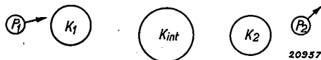
Fig. 7. Diagram of a nuclear reaction resulting on the bombardment of a nucleus K_1 with a projectile P_1 , as a result of which an intermediate nucleus K_{int} is produced, which then disintegrates into a new nucleus K_2 and a projectile P_2 .
