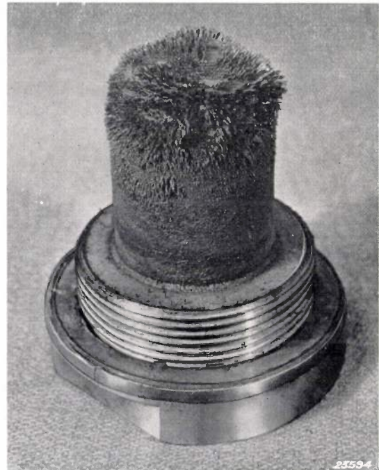
Fig. 6. Oil filter magnet covered with iron filings.
