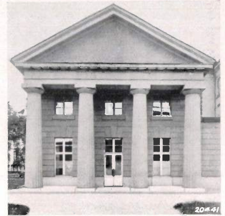
Fig. 2. (Right) The same building when seen in diffuse daylight loses all plasticity in its finer profiles and hence the characteristic appearance which the architect had intended.
