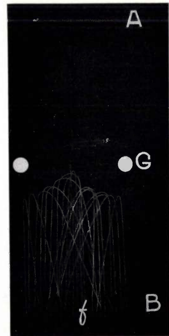
Fig. 8 a - f. Photographs of paths of balls, obtained by shooting a parallel "beam" of balls (in the arrangement of fig. 3) with a constant velocity perpendicular to the line joining the grid supports. The different figures are obtained by taking the height of G successively a little greater.
