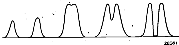
Fig. 6. Variation of the anode current of a three-electrode valve with sinusoidal excitation voltage (increasing from left to right). If the excitation voltage is so high that the anode voltage drops below the grid voltage at the peak value of the anode current, the greater part of the emission current passes to the grid at the expense of the anode current. This produces a trough in the current curve of such character that the first harmonic of the anode current no longer increases above a certain excitation voltage.
